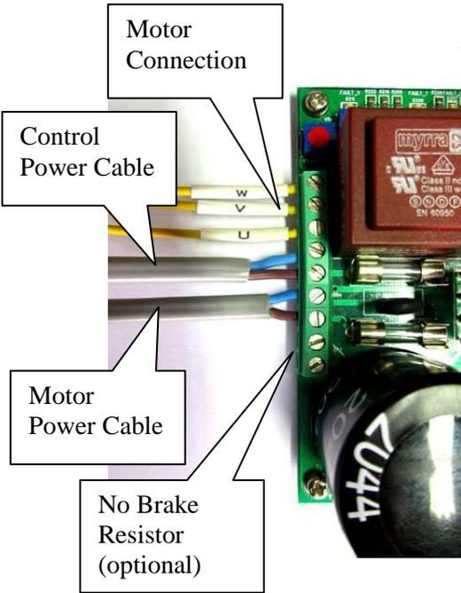
Fig. 5. Separate "Motor Power" and "Control Power".
