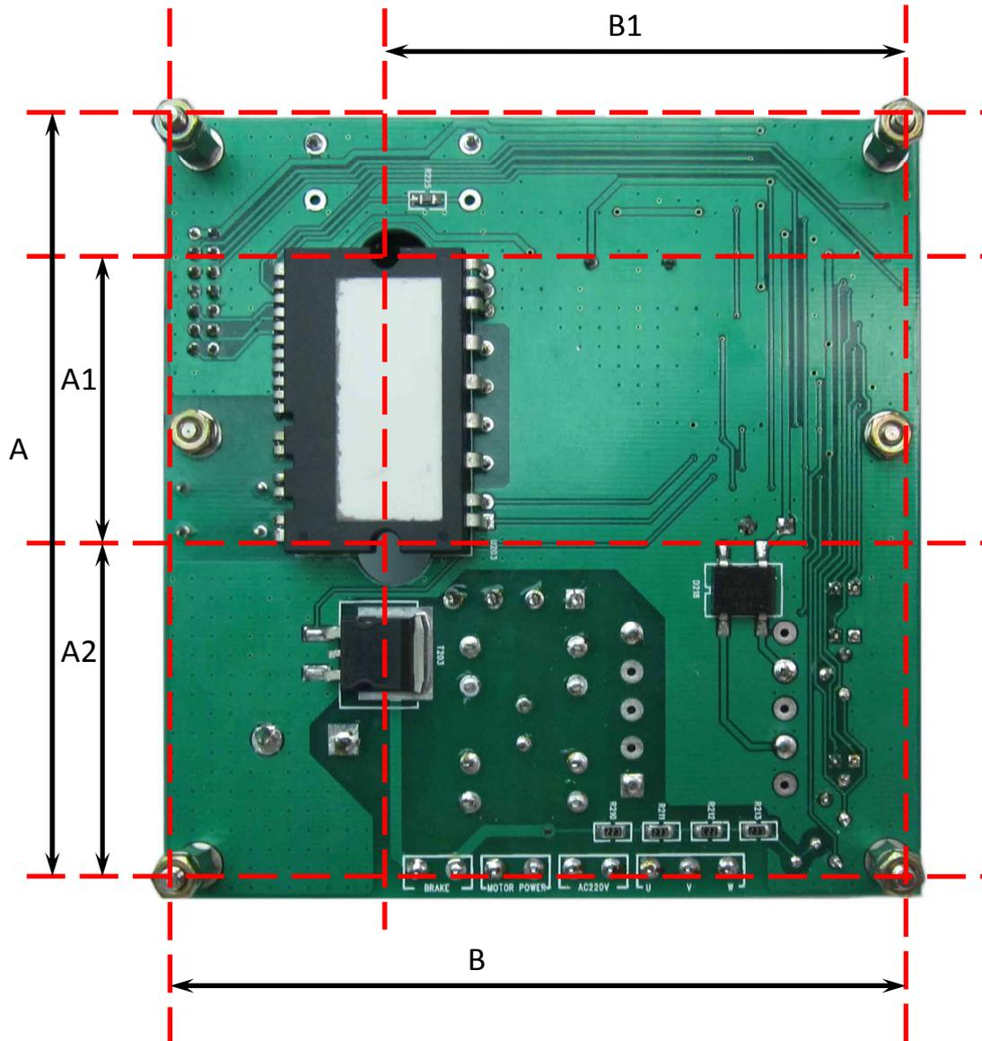
Fig. 3. Mounting holes location
